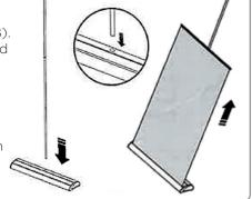
7. Insert the hook of the pole into the rear slot of the top bar, which is marked by a sticker.
